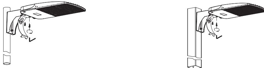
Note: When installing on a round pole, please remove the prominent rubber gasket as shown in figure. Just keep flat rubber gasket for installation.
