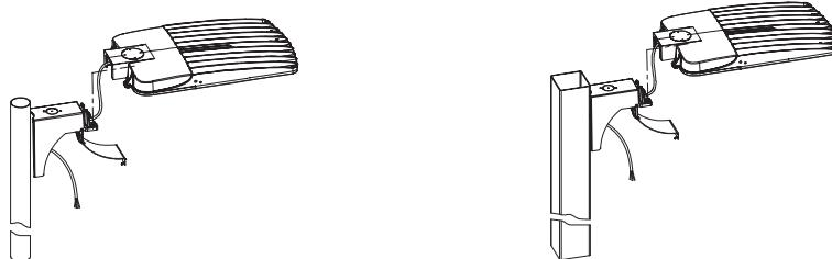
Step 4: Hang the fixture on Pole Mount bracket, lock the fixture by tightening screws through bracket with allen wrench.
